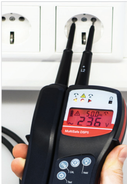
One-hand operation for testing sockets
